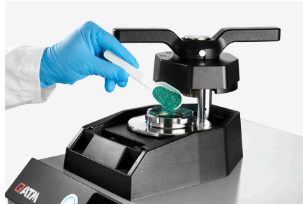
2. Fill in mounting resin
