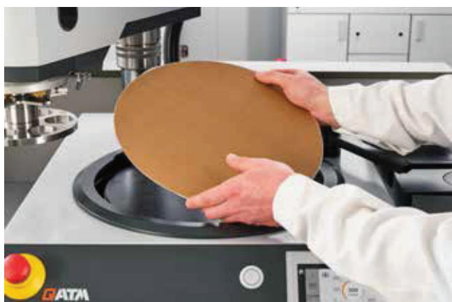
Applying GALAXY X-Tap on magnetic foil
