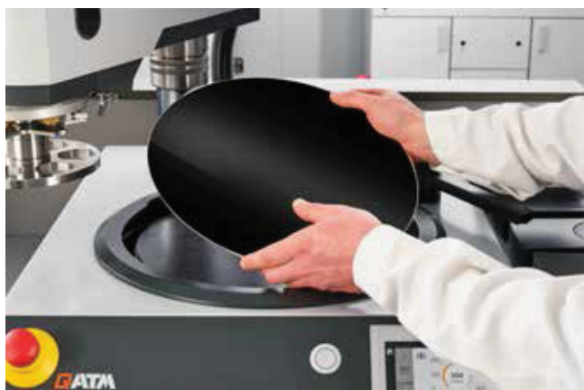
Applying GALAXY Quick-Tap on magnetic foil
