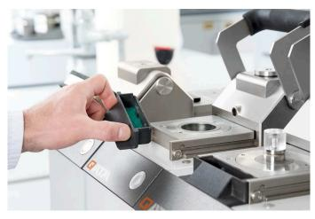
3. Clean dirt trap as excess mounting material is automatically pushed towards it
