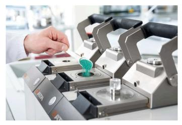
1. Fill the mould with the respective mounting material
